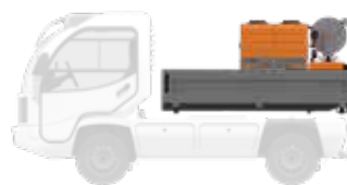
water tank, brine spraying system
